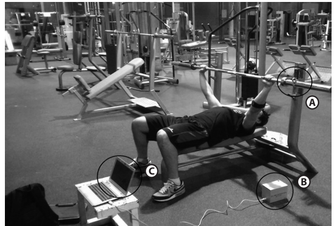
Figure 2. A. Connection between the bar and the linear transducer; B. Linear transducer; C. Laptop.
