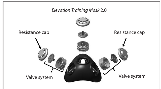
Figure 1. Elevation Training Mask 2.0 resistance caps and valve system
